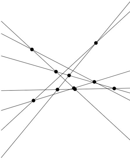
(c) The marked intersections form a vertex cover of the  $\mathcal{H}_{vertex-cell}$  hypergraph: every cell has at least one such intersection on its boundary. That is, these vertices *guard* the cells.
