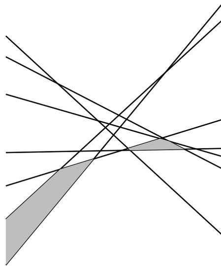
(d) The two marked cells form a vertex cover of the  $\mathcal{H}_{cell-zone}$  hypergraph: every line has a segment that lies on the boundary of one of these cells. That is, these two cells *guard* the lines.
