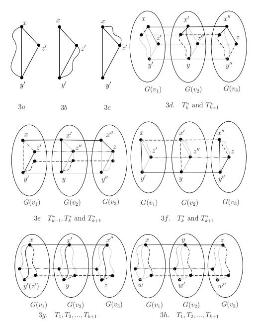
Fig. 3: The edges (or paths) of a tree are shown by the same type of lines. The lightest lines stand for edges (or paths) not contained in  $T_i^*$ .
